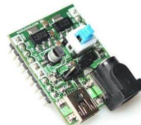
**NOTE!** Connection of two voltage sources may damage the circuit. When connecting the USB cable, please disconnect the DC cable and vice versa.
