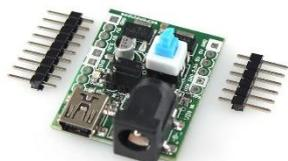
*The module supplies the voltages of +3.3V and +5V. The built-in ON/OFF switch makes control easier. A USB or DC connector from the power supply with the voltage of up to +12V can be used for supply.*
