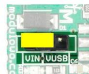
**Note!** VSEL Jumper is used to set the power supply module. The module can be powered from the USB connector or VIN connector.
