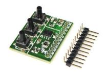
This controller enables independent control of two model servomechanisms using buttons or 1/0 signals. The leads are ideal for servo signals (SYG, +V, GND), so there is no need to use additional wires or adapters.
