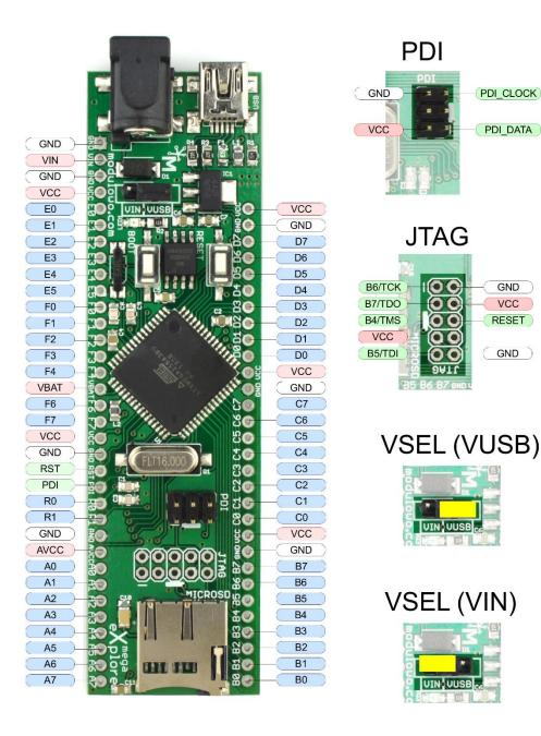
**Note!** VSEL Jumper is used to set the power supply module. The module can be powered from the USB connector or VIN connector.
